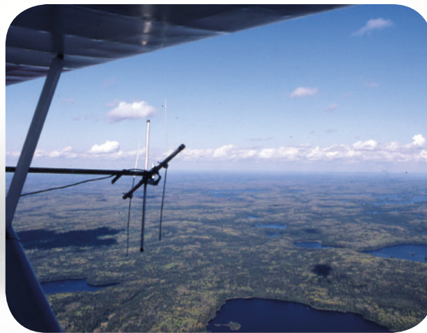
A directional, animal radio-tracking antenna mounted on each wing strut of an airplane allows a biologist with a special receiver to home in on radioed animals.
